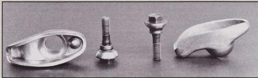
Rocker arm designs were compromises partially dictated by the head’s unique combustion chamber, valve and pushrod layout. These arrangements were concessions to a plan to retain the B-wedge head bolt pattern. Although the rocker ratio measures 1.60:1, the pushrod angles and odd rocker geometry result in an effective 1.58:1. During development, there were concerns that
