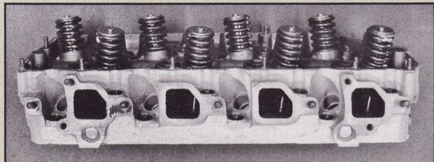
The exhaust ports have unique “modified-D-shaped” exits. Efforts to fit a centrally located sparkplug into the combustion chambers resulted in the use of a “peanut-style” sparkplugs having a 5/8” hex rather than the 13/16” size; these have become commonplace nowadays. For wrench clearance, some of the 7/16” head bolts along the foot-section row use smaller (5/8” rather than 3/4”), hex heads. Note I-E-I-E-I-E-I-E pattern which is better for exhaust cooling.
