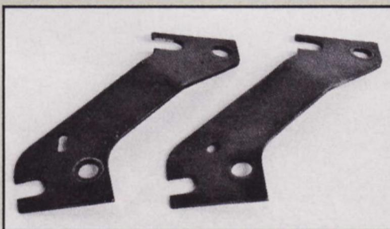
*Making their first appearance on a Chrysler V8, stamped-steel guideplates help position the pushrods' tops and align them with the rockers. They also helped guide the rockers' travel through the arcs prescribed by the valves' compound angles.*
