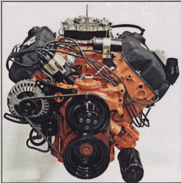
From the appearance of all these finished castings and special stampings, the motor was well on its way to production. Engineers anticipated that the Ball-Stud Hemi arrangement would have been both less costly to produce and lighter in use. A Ball-Stud Hemi would also “come down the line better” and would fit more production car bodies with fewer plant problems than the physically larger Street Hemi.
