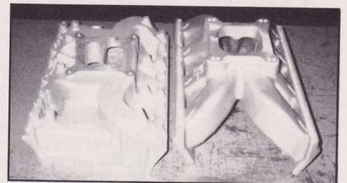
5. The difference between the Indy Cylinder Heads Spider single-plane and the Mopar Performance M1 dual plane is obvious. Arruzza will supply an HP499 with your choice of any Hemi manifold.
