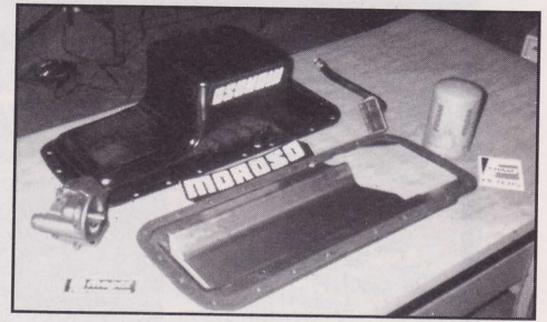
2. The oiling system is pure simplicity in its execution. A baffled 8-quart pan and 1/2-inch pickup from Moroso, a high-volume/high-pressure pump and windage tray from Mopar Performance, and a Fram HP1 filter is all there is to it.
