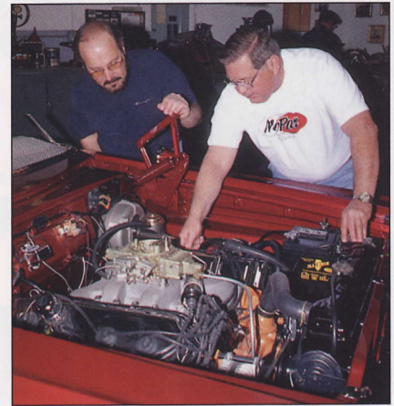
Tom Moshis (left) and Bill Petrow, of engine parts supplier Special T's Unlimited, inspect the 426-cid Hemi placed in the restored Charger show car.
